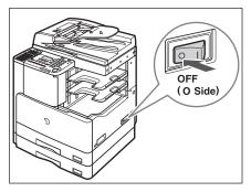
$\hfill\square$  Disconnect the power cord from the wall outlet.
