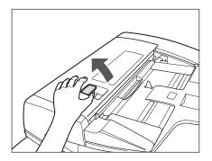
**2** Clean the rollers (a total of three places) inside the feeder cover with a cloth dampened with water. Then wipe the area with a soft, dry cloth.
