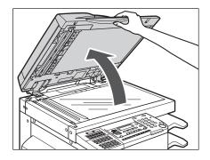
**9** Clean the feeder scanning area (the left side of the platen glass) and the document feeding roller, with a cloth dampened with water. Then, wipe the area with a soft, dry cloth.
