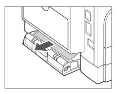
${m 3}$  Pull out the paper drawer and remove any jammed paper.
