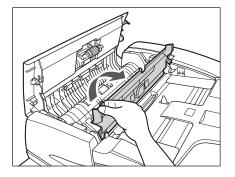
**4** Clean the rollers (a total of three places) inside the inner cover with a cloth dampened with water. Then wipe the area with a soft, dry cloth.
