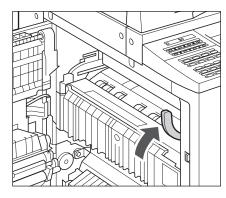
**6** Place your hand where the hand symbol is located on the left cover of the main unit, and then gently close the left cover until it clicks into place in the closed position.
