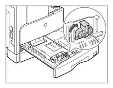
**5** Lower the lock lever to the left to lock the side guide.
