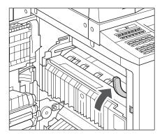
7 Place your hand where the hand symbol is located on the left cover of the main unit, and then gently close the left cover until it clicks into place in the closed position.
