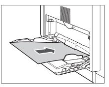
When you use the stack bypass to make copies, straighten out curled paper prior to use, as shown below. Curled paper may cause a paper jam.
