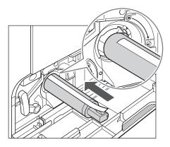
**6** Hold the toner cartridge with one hand, and remove the seal by pulling it out with the other hand.
