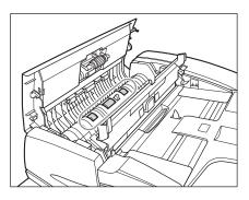
**5** Clean the transparent plastic part of the inner cover with a cloth dampened with water. Then wipe the area with a soft, dry cloth.
