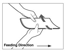
If there is difficulty in straightening out curled paper, curl the front edges of the paper upward, as shown below.
