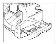
10 Gently push the paper drawer back into the machine until it clicks into place in the closed position.
