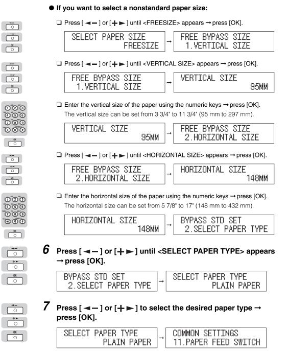
The standard size and type for the stack bypass is set.
