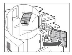
**2** Pull out the staple case, holding the tab as illustrated below.
