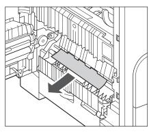
**4** Pull out the paper drawer and remove any jammed paper.
