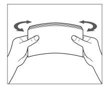
Place the envelopes on a clean, level surface, and press all the way around the envelopes by hand, in the direction of the arrows, to remove any curls. Repeat this step five times for each set of five envelopes.
