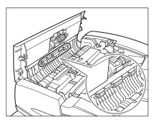
${m 3}$  Open the inner cover, holding it by its front tab.
