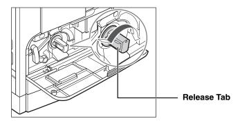
${f 3}$  While pushing down the release tab, pull the toner cartridge out in the direction of the arrow in the illustration below.
