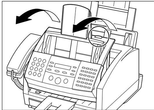
3. Hold the cartridge by its handle and remove it as shown.
