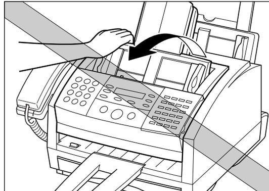
2. Hold the cartridge by its handle and remove it from the machine.
